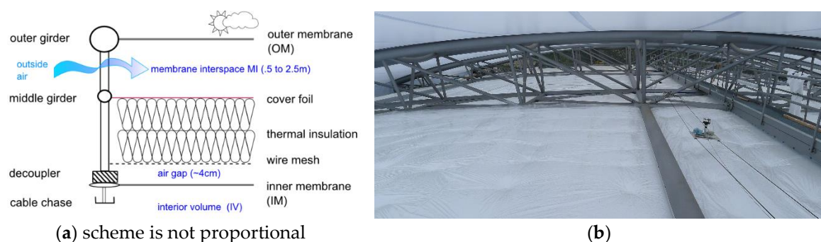
Figure 3. (a) Side view scheme of the roof layer construction; and (b) photograph of the membrane interspace. A monitoring platform for other measurements is visible on the two ropes on the right-hand side of the image.
