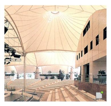
The cover had, in each of its cones, vents **that** evacuated **the hot air** that was stored in them. Despite this, the cover reached an average temperature under the design conditions of 45°C. Seeing that the comfort temperature was 26 degrees for the external area and 22 degrees for the stage area, it was seen that it was essential **to treat the cover by irrigation**. In this way, the cover was cleaned, which prevented the temperature of the cover from increasing due to dirt.
