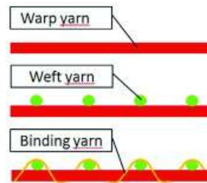
Figure 15. Three independent thread systems of TransProof.
