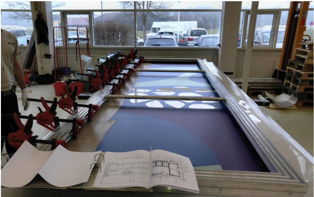
Figure 10: Assembly of the 64 frames in Taiyo Europe's workshop (standard size 4.2 x 1.3 m, as shown here; special size 4.2 x 0.5 m)
