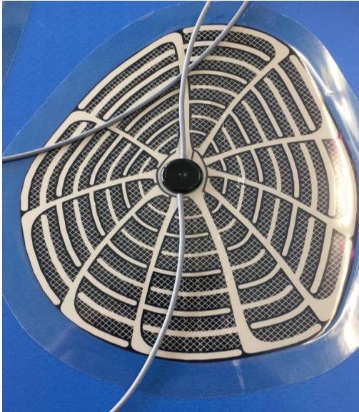
Figure 11:OPV-modules glued on the backside
