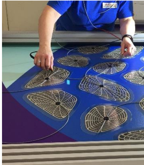
Figure 12:Connecting the OPV-modules
