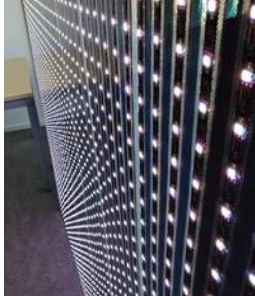
Figure 6: Prototype of the ETFE-MFM module, here with LED switched on (uniform white light) [1]
