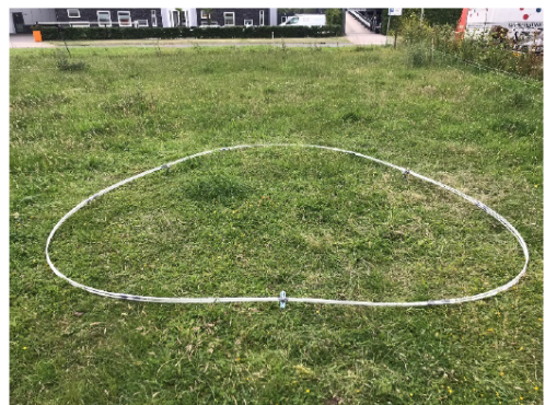
Figure 6: GFRP rings with 3 ground anchors (left), GFRP rings connected to ground anchors (right)
