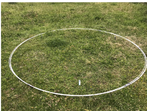
Figure 6: GFRP rings with 3 ground anchors (left), GFRP rings connected to ground anchors (right)
