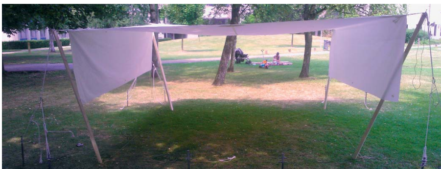
Figure 2. Prototype 1 forms a saddle shape with two high and two low points
