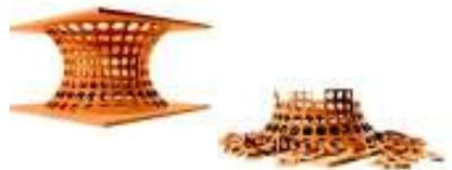
Figure 13. One full catenoid rotated in space. A compression-only form and a self-interlocking produce a simple joining through stacking.
