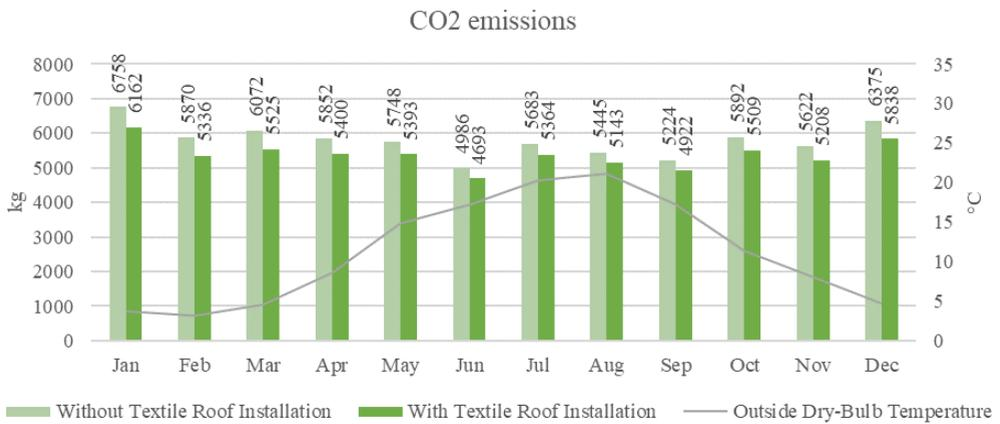
Figure 4: Chart showing the CO2 emission levels in the building during 12 months without the textile roof installation and with it.
