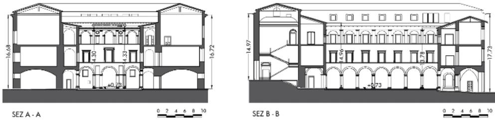
Figure 2: Transversal (left) and longitudinal section (right) of the building.
