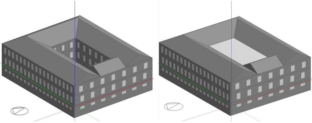
Figure 4: Design Builder model of the building without the ETFE courtyard covering (left) and with the ETFE courtyard covering (right).
