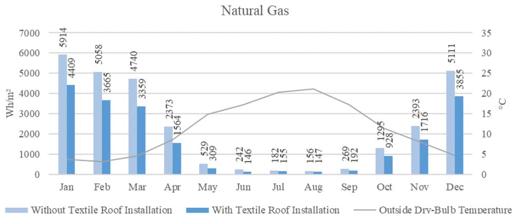
Figure 6: Chart showing the Natural Gas consumption levels in the building during 12 months without the textile roof installation and with it.
