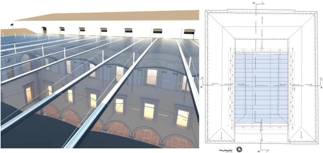
Figure 3: Rendered image of the ETFE roof seen from the top (left), installation of the ETFE roof (right).
