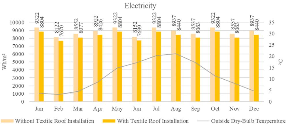
Figure 5: Chart showing the Electricity consumption levels in the building during 12 months without the textile roof installation and with it.
