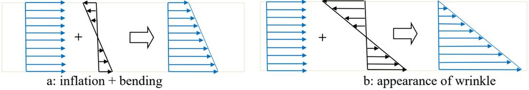
Figure 4: longitudinal stresses in the membrane
