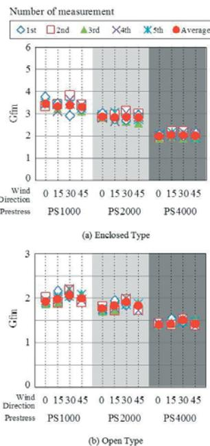
Figure 12.  $G_{fm}$  depending on pre-stress and wind direction on each model type
