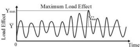
Figure 1. Time variation of load effect by dynamic action of wind
