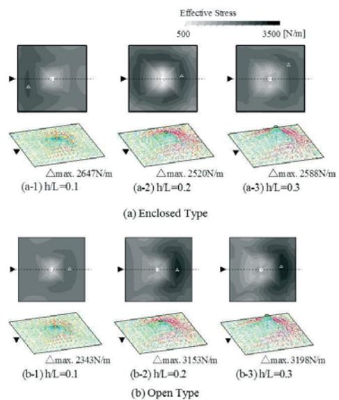
Figure 9. Effective stress and maximum value of it when the wind velocity pressure  $q$  is 455N/m<sup>2</sup>.
