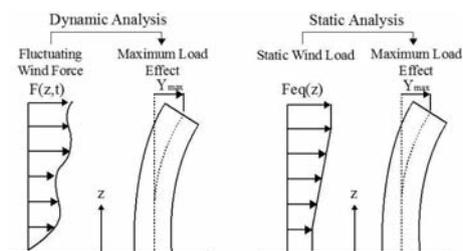
Figure 2. The concept of effective static wind load
