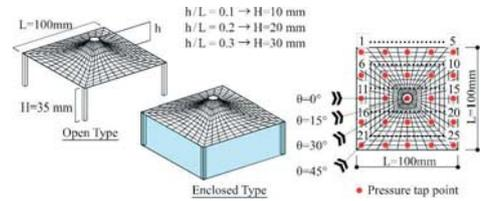
Figure 5. The outline of models; two types model was prepared, namely "open type" and "enclosed type", and there are 25 pressure taps on the roof in each model.
