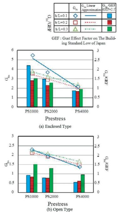
Figure 13.  $G_{fm}$  for the design wind load and comparison with gef of the building standard low of japan ( $gef=2.5$ )
