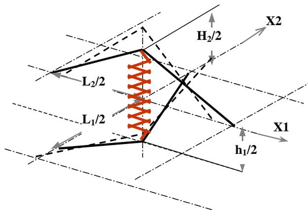
Figure D-2 Triangular model with a spring in the knot [Bög04]
