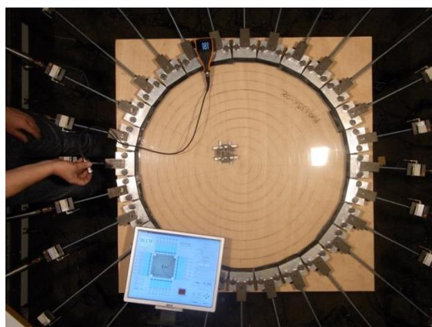
Figure B4-11 Circular sample in biaxial testing machine [© DEKRA/Labor Blum]
