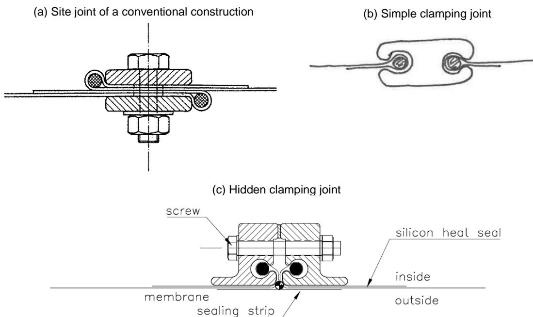
Figure 8-3 Typical exemplary clamped (bolted) membrane joints with metal plates, bolt ropes and bolts according to [1<sup>st</sup> row, left: Bub97, 1<sup>st</sup> row right: © M. Nieger, 2<sup>nd</sup> row © formTL]
