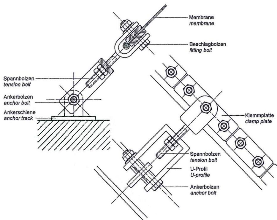
Figure 8-9 Edge element made of rotating metal fitting and tension bolt modified according to [Bub97]
