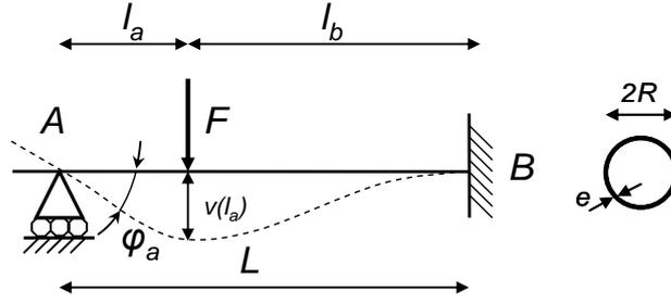
Figure F-5 Propped cantilever beam with a single point load
