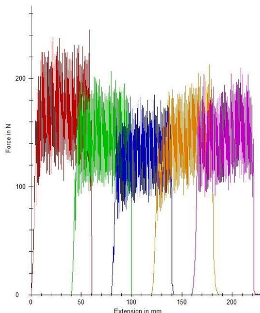
Figure 2-6 Typical results of a tear test [© ELLF]
