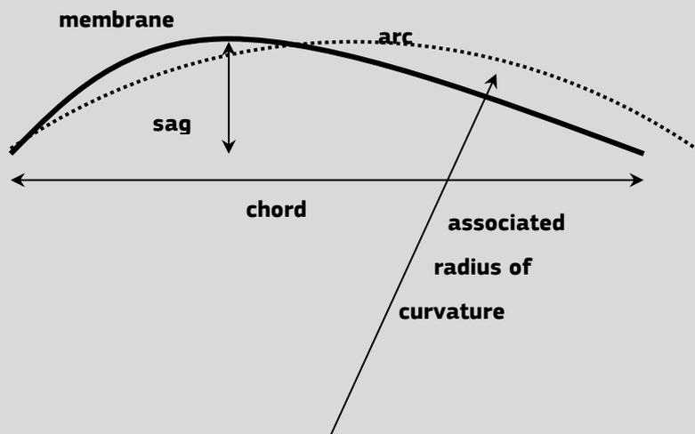
Figure 3-2 Membrane and associated arc
