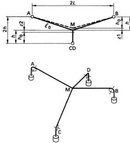
Figure 3-6 Model of the bi-cable [ML93]
