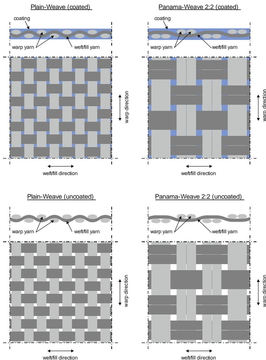
Figure 2-2 Most common weaving constructions for fabrics used in textile architecture
