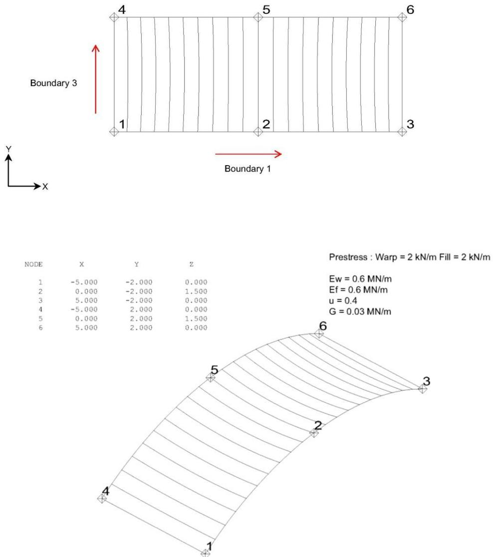
Figure E-5 Model 5 – Barrel Vault 1 Factored analysis review [© N. D. Gibson, TENSYS]
