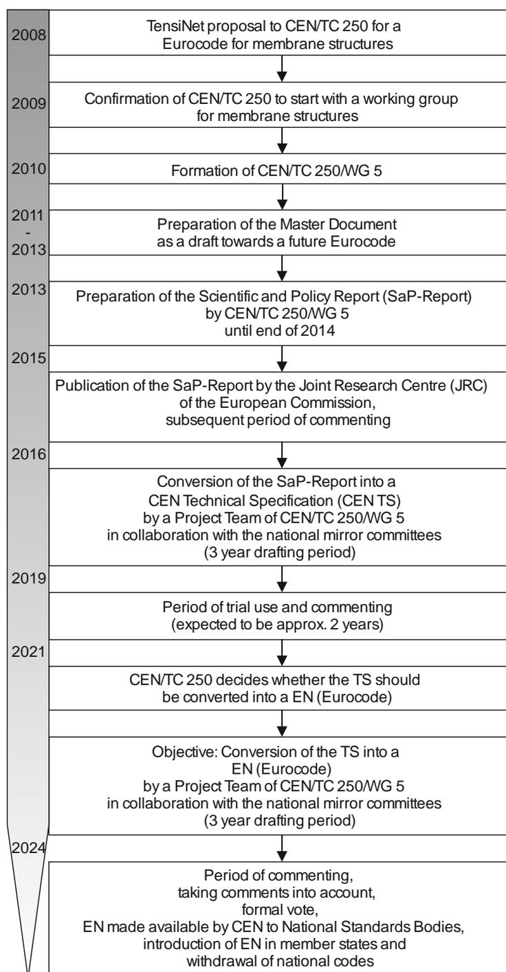
Figure 1-3 Steps to a Eurocode for Membrane Structures [SUMG14]
