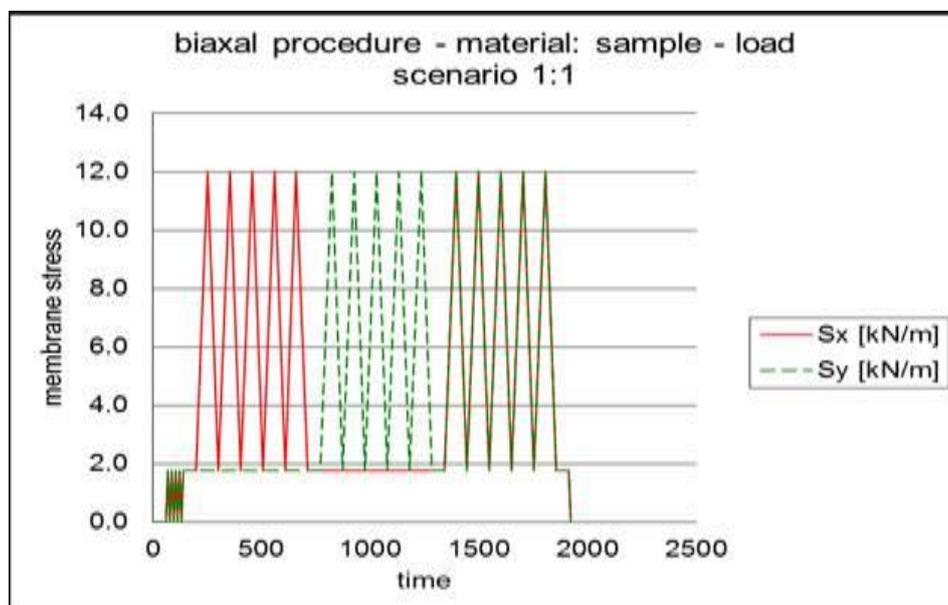
Figure B4-7 Biaxial load scenario 1:1 [© formTL]
