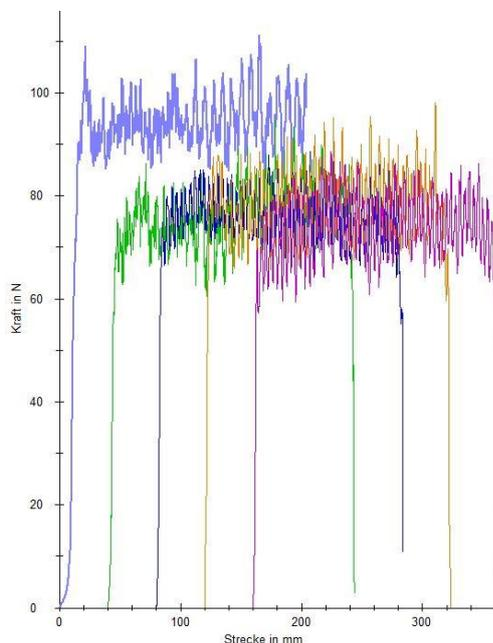
Figure 2-8 Typical results of an adhesion test [© ELLF]
