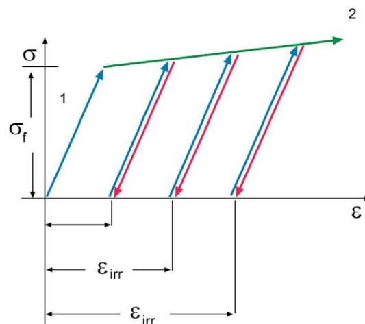
Figure 7-7 Idealised stress-strain curve [© DEKRA/Labor Blum]
