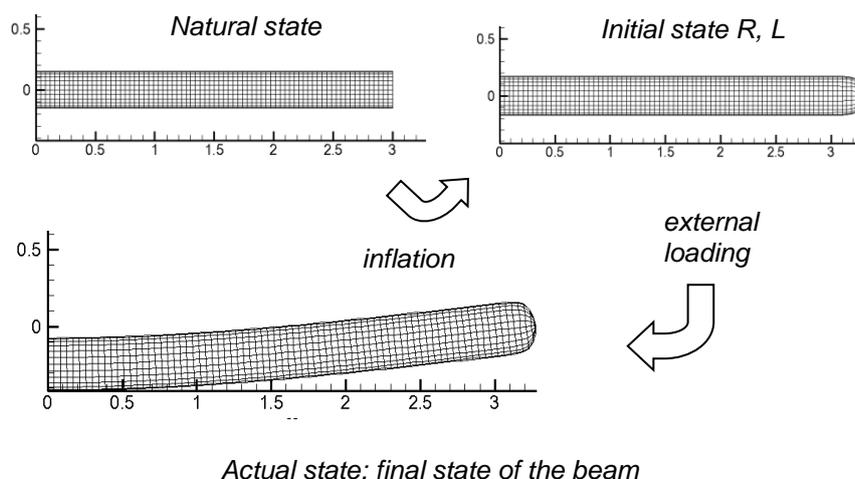
Figure 5-14 The three states for an inflated beam (source and ©: J.-C. Thomas)
