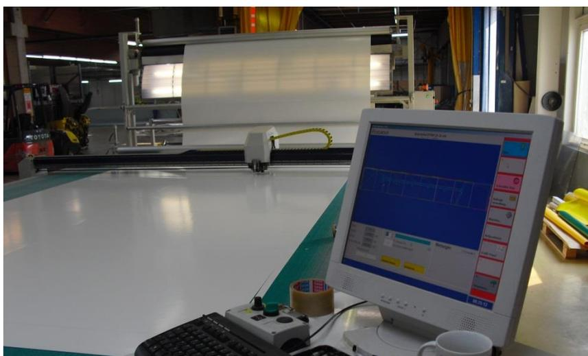
Figure 9-1 Automatically cutting of membrane material via electronic data files
