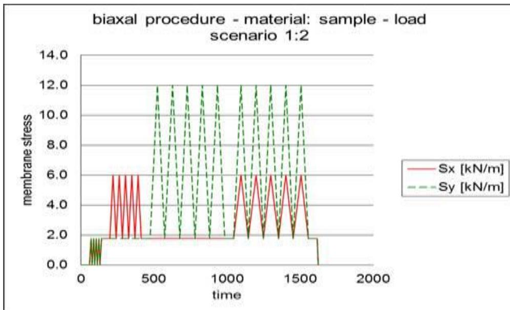
Figure B4-9 Biaxial load scenario 1:2 [© formTL]
