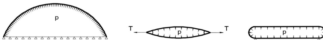
Figure 1-16 Air halls (left), cushion (middle) and air beam (right) [© M. Mollaert]
