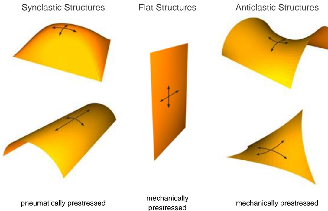
Figure 1-2 Typical shapes of membrane structures [US13a]
