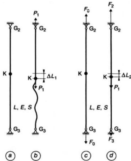
Figure 3-4 Model of the colinear cables [Lau92]
