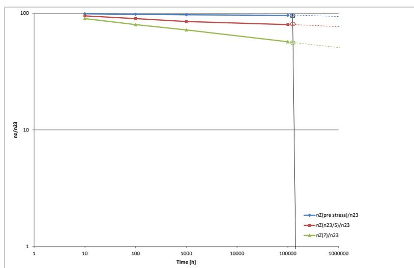
Figure C3-2 Residual strength of strips under constant load (3 load levels) over time (at 23°C and 70°C), logarithmic scale [© DEKRA]
