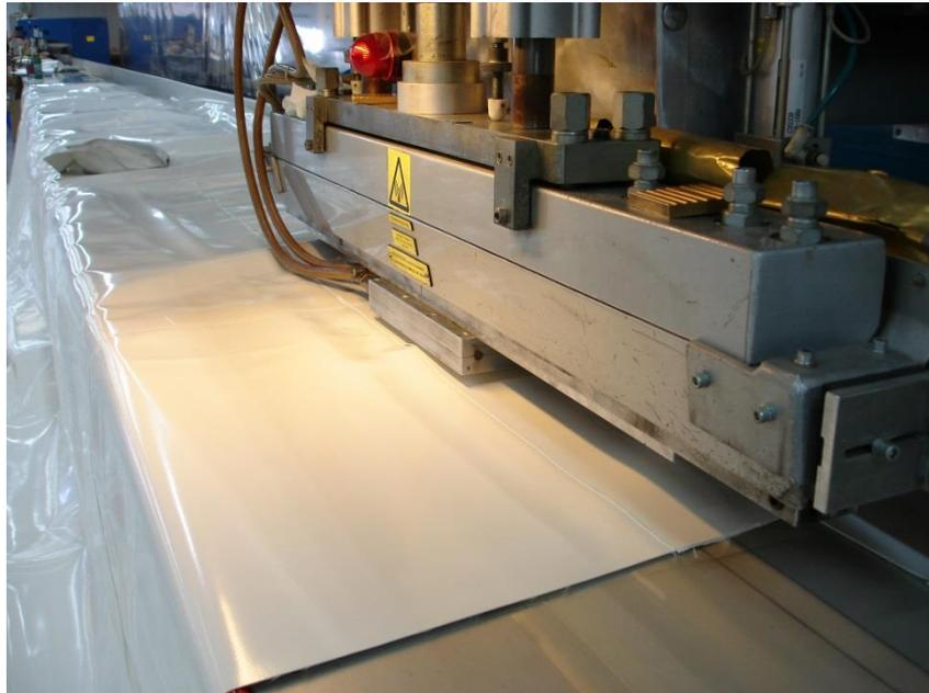
Figure 9-2 Typical welding situation [© CENO Membrane Technology GmbH]
