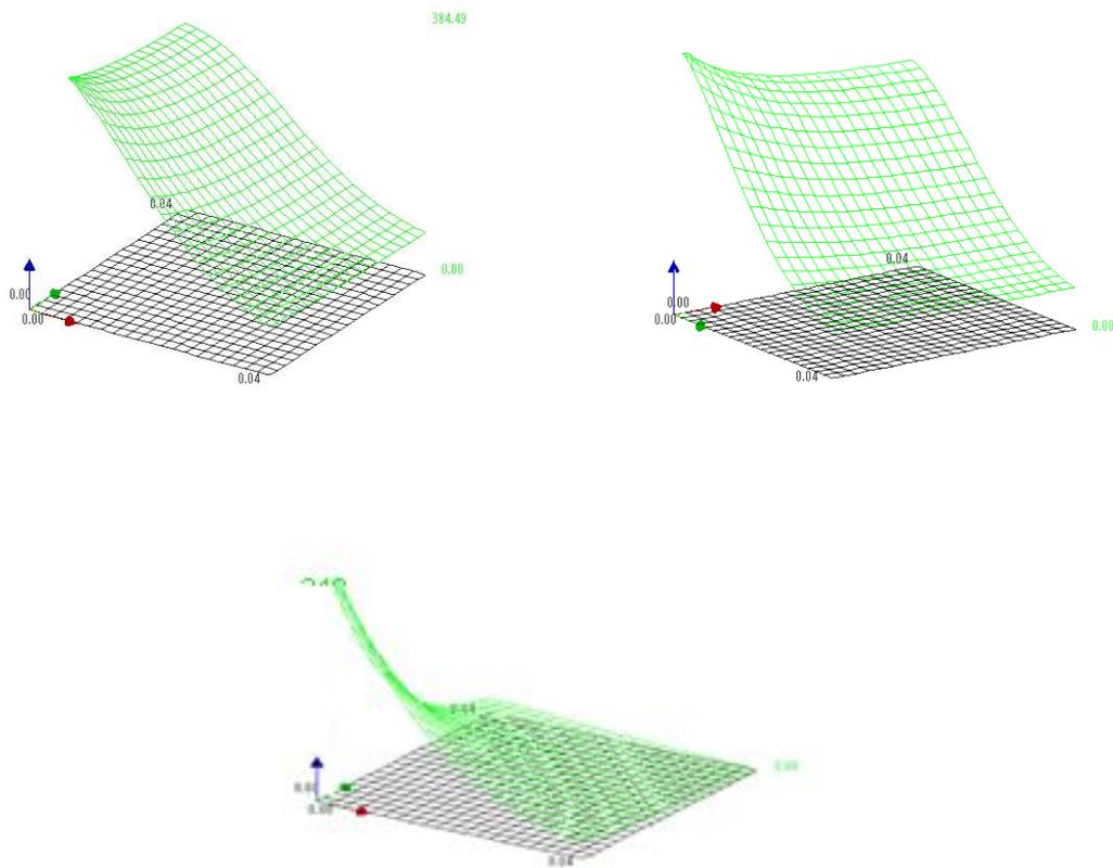
Figure D-4 Elastic Modulus (z-axis) in warp direction  $E_{1111}$  (left hand above), in weft direction  $E_{2222}$  (right hand above) and interaction between warp and weft direction  $E_{1122}$  (below) in dependence of the elongations in warp and weft (respectively stresses in warp and weft) [© Bögner-Balz]
