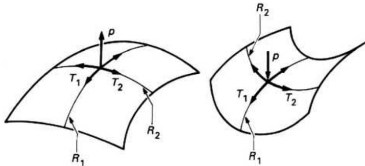
Figure 3-5 Local Equilibrium of a tensioned membrane
