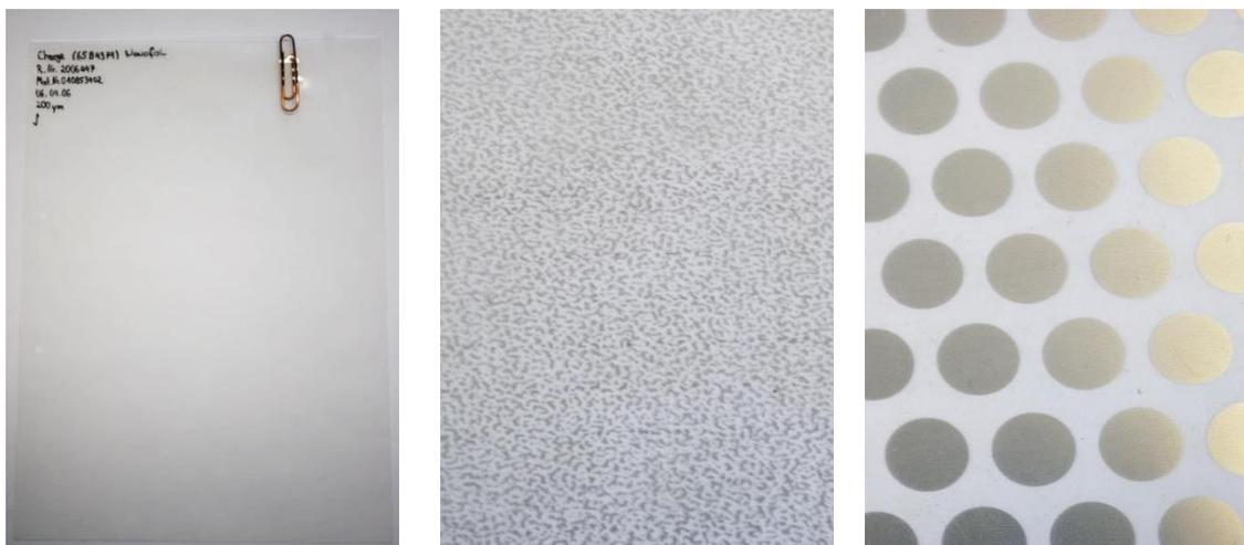
Figure 2-9 Exemplary plain and printed ETFE-foils [© ELLF]
