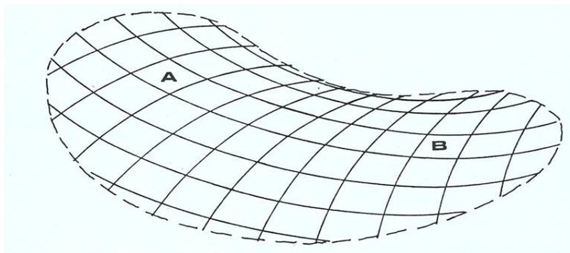
Figure 1-11 Anti-clastic surface [© M. R. Barnes]
