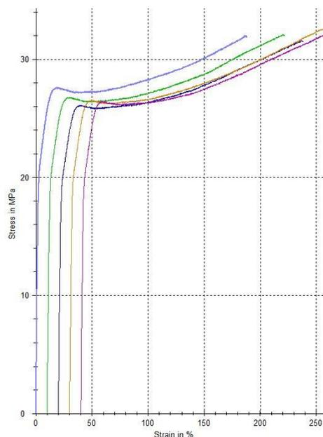
Figure 2-10 Tensile test specimen (here: ETFE-foil edge detail), left, and typical stress-strain-diagrams for ETFE-foils [© ELLF]
