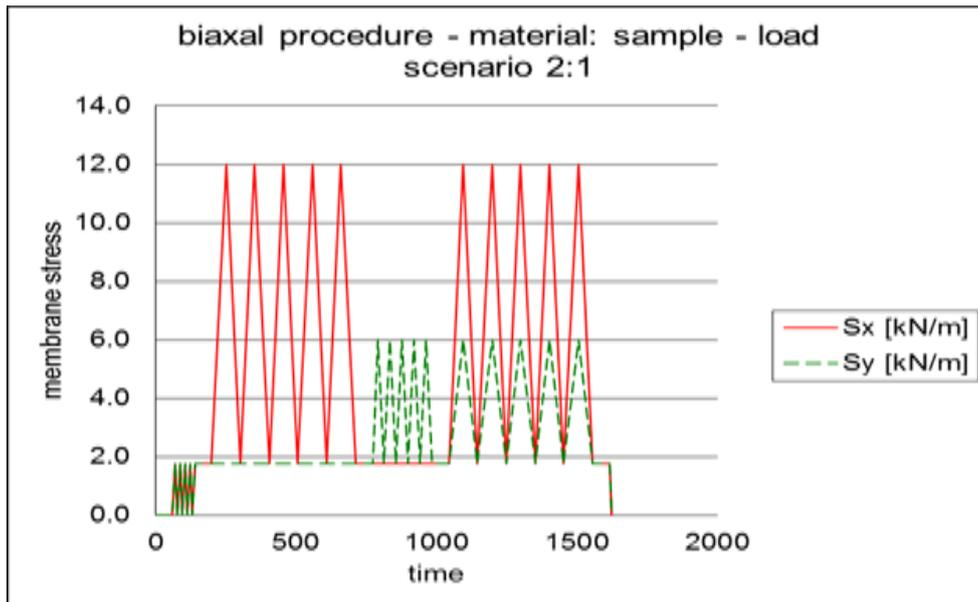
Figure B4-8 Biaxial load scenario 2:1 [© formTL]
