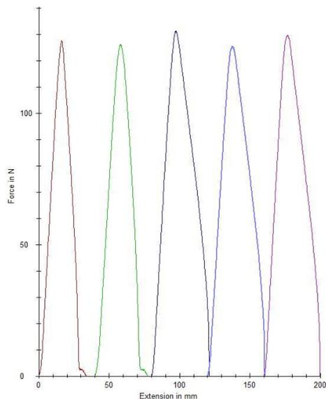
Figure 2-11 Typical force-extension-diagrams for ETFE-foils [© ELLF]
