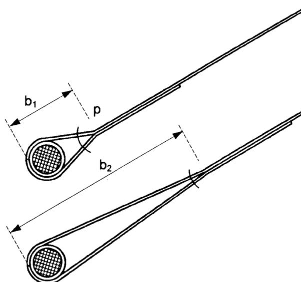
Figure 8-7 Different widths of membrane pockets [Bub97]
