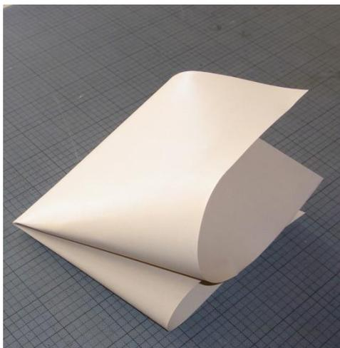
Figure B2-5 Procedure to create a running crease, specimen folded twice [© DEKRA/Labor Blum]
