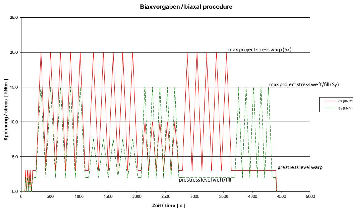
Figure B4-6 Load scenario for a modified biaxial test according to formTL [© formTL]
