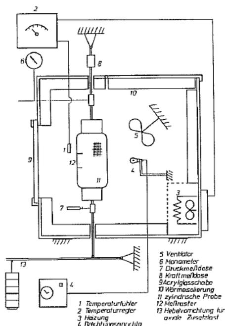
Figure C2-1 Test equipment for biaxial loads (principle sketch) [Meff78]
